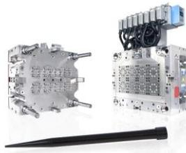
**Image 2:** Each männner mould cavity cluster comprises eight removable and replaceable cavities, a hot runner nozzle head with eight individual heat controlled nozzle tips and eight floating core pilot bushings.
