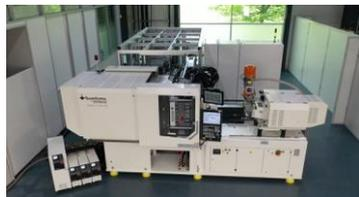
**Image 1:** The full turnkey IVD production cell is capable of mass producing 320 million individual IVD components per annum
