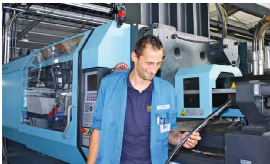
Sasa Grbesa with one of the chrome strips, standing in front of an Ergotech 650 system on which the components were produced.
