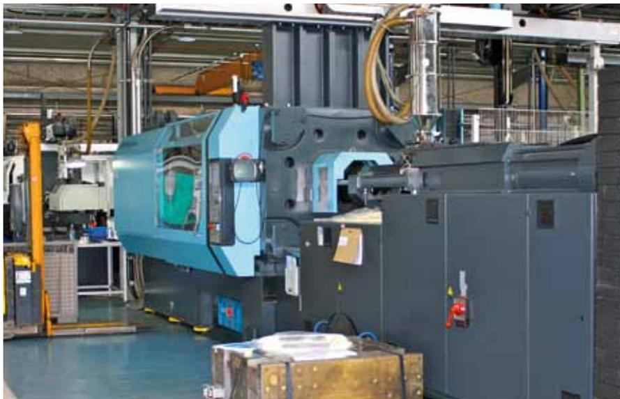
BIA currently operates a total of 43 injection moulding machines for 1-, 2- and 3-component technologies, most of which are from Sumitomo (SHI) Demag.
