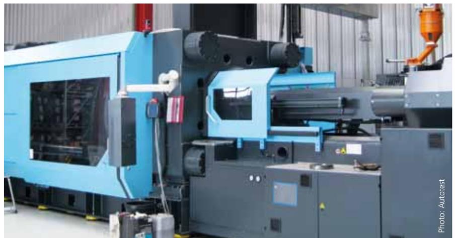
Large machine for large components: The holding frames of the bumpers of the Porsche Panamera are produced on the System 1500 injection moulding machine from Sumitomo (SHI) Demag with 15,000 kN clamping force.
