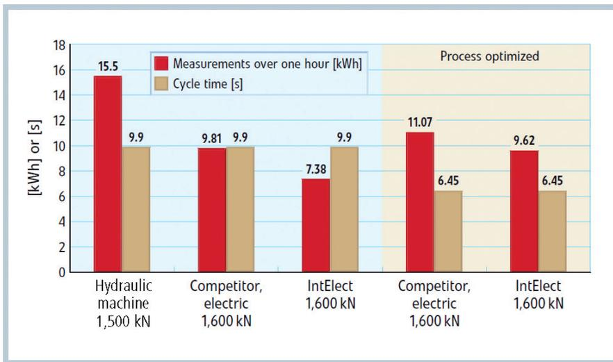
Fig. 1. Comparison of energy consumption between a hydraulic machine 150 t, an electric IntElect 160, and another electric machine. Process optimization (measured values right and second from right) reduced energy consumption and increased outputs
