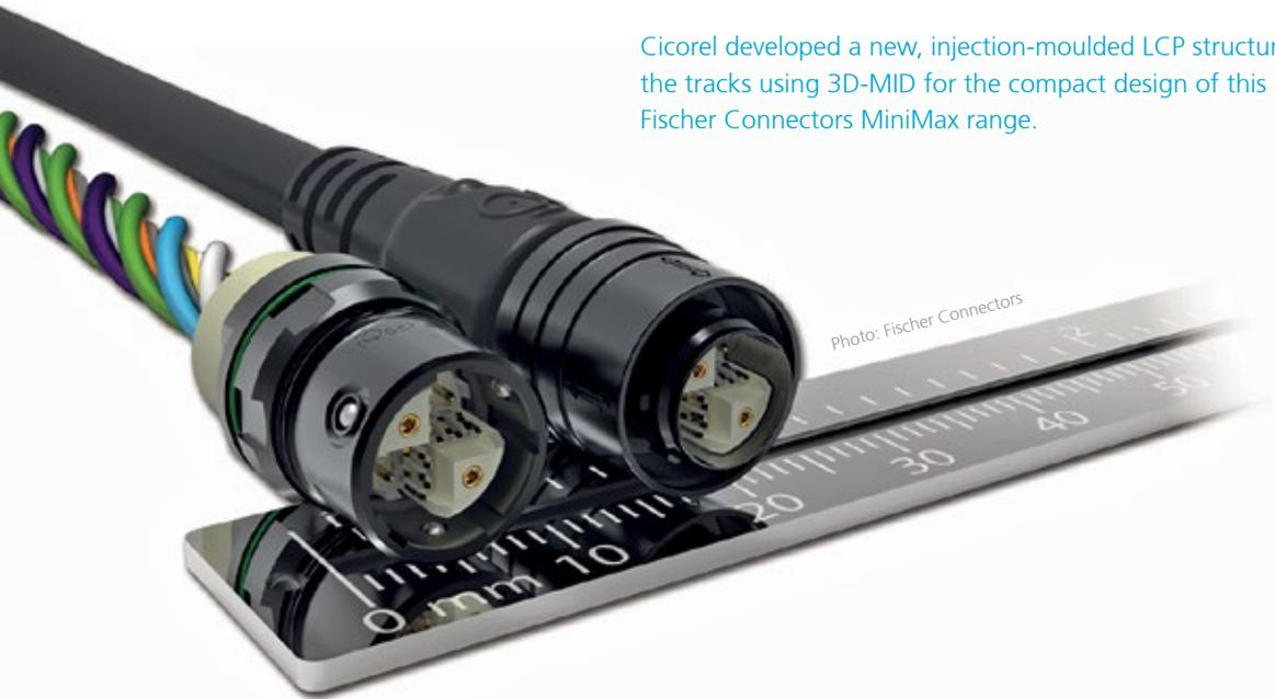
Cicorel developed a new, injection-moulded LCP structure for the pins and created the tracks using 3D-MID for the compact design of this plug connector from the Fischer Connectors MiniMax range.
