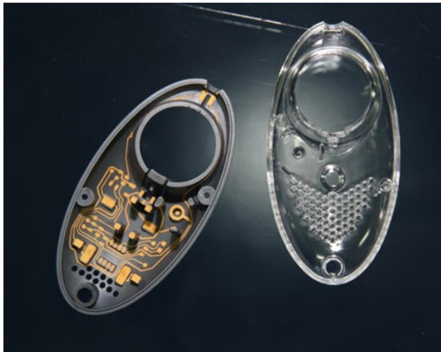
aerials in hearing aids. Conventional aerial technology can be replaced by 3D-MID which can create the appropriate structure directly on the housing in a very space-saving manner. Once painted over, the structure is functional but no longer externally visible.
