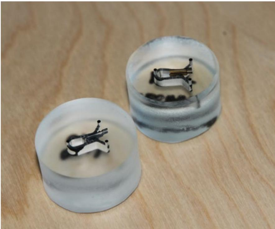
Using a number of sections, the surface quality of the materials is examined as this has a major impact on the subsequent laser structuring.
