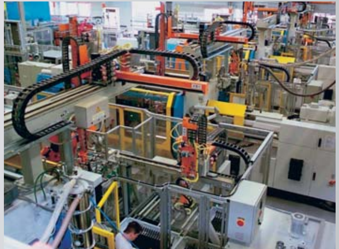
Production shop with System machines 5,000 kN for the production of automotive parts
