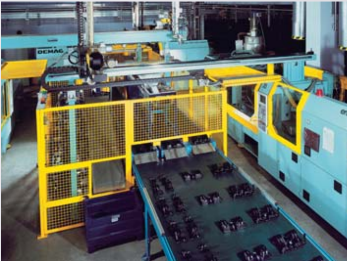
Production cell incorporating System machines producing intake manifolds
